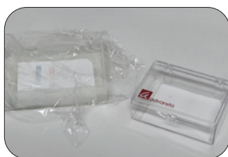
Save antibody and buffer by using the smallest tray that can hold your blot
